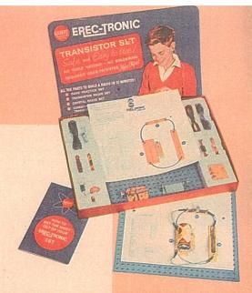
erectronic transistor set—All the parts to build a working radio in just 10 minutes! Needs no tools, solder. Printed templates on pegboard show where parts go; place where indicated, hook 'em up and set is complete! Includes crystal diode, 250 mmfd. capacitor, code sending key and more. Instructions. 8 to 16 yrs.
